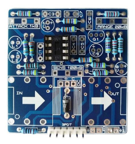
First of all place the IC sockets (without the ICs). Pay attention to the orientation! The small notch in the socket should be oriented as indicated in the PCB.
