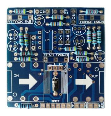
Place the resistors and diodes. If you have troubles reading the values, check out our "Reading Part Values" tutorial.
